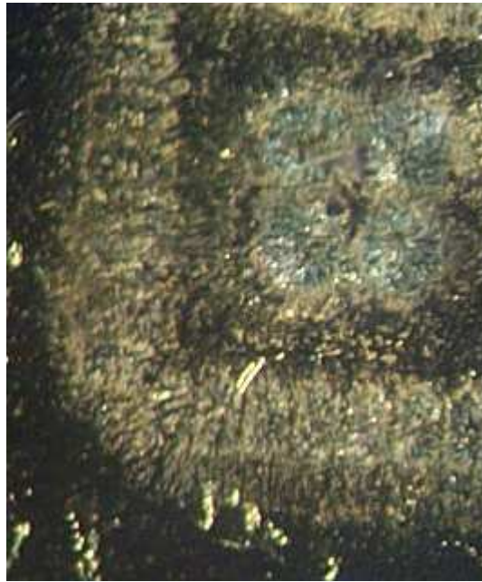
Figure 21 Base plate shows no significant signs of wear due to socket
