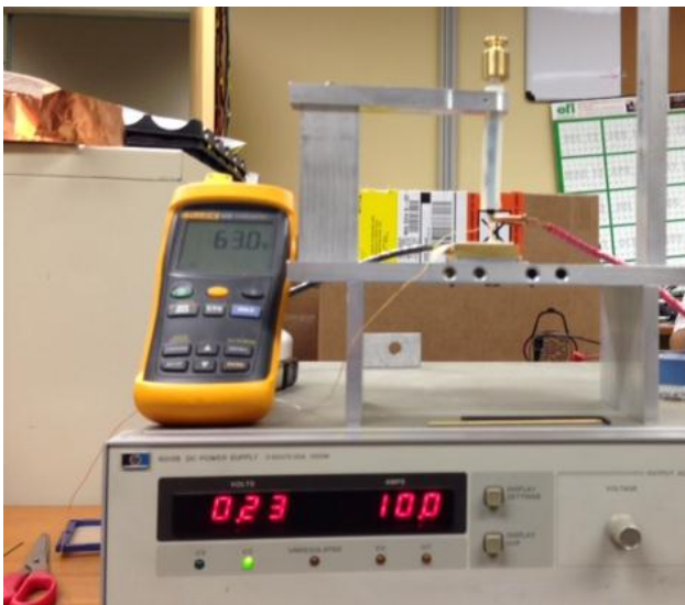
Figure 1 – Test Setup 10 amps 40 C° rise in temperature
