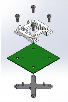
Underneath the DUT board is a support plate that is secured to the base plate to prevent bowing.
