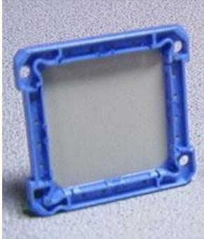
A stretch frame holds the PariPoser<sup>®</sup> material taut and makes it easy to position the contactor into the socket.
