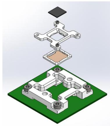
This exploded view shows the wafer, the alignment plate, the stretch frame with the PariPoser<sup>®</sup> material, and the base plate. The stretch frame with the contact material can be easily removed if worn or if contaminated by the solder.
