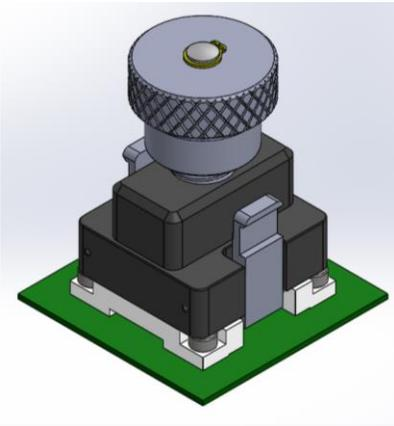
The assembled socket has a load-adjustment knob to apply the correct pressure to the wafer. The clips on the side keep the cover mounted to the base plate.
